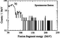
FIG. 1. (a) Total beam-on and beam-off  $\alpha$ -particle energy spectra of events registered by the focal-plane detector and by both the focal-plane and side detectors in the reaction  $^{242}$ Pu+ $^{48}$ Ca. The solid histogram shows the energies of events observed during beam-off periods in the correlated decay chains (see Fig. 2 and Table II). (b) Total fission-fragment energy spectrum; the solid histogram shows the energies of events observed in the correlated decay chains.
