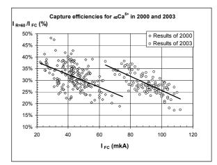
Figure 5: The  ${}_{48}Ca^{+5}$  ion capture in acceleration efficiencies before (2000) and after (2003) the injection modernization
