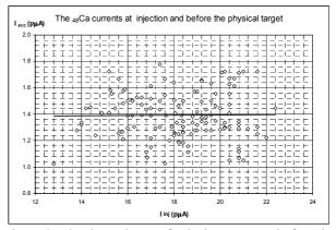
Figure 3: The dependence of  $_{48}$ Ca ions current before the physical target ( $I_{acc}$ ) on injected one ( $I_{ini}$ ) in 2003.
