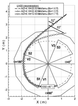
Figure 4: The scheme of the ion beam extraction by deflector in two extraction regimes
