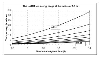
Figure 2: The energy range of possible accelerated ions
