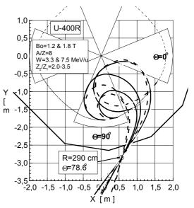
Figure 5: The scheme of the ion beam extraction by stripping foils with two separate foil probes. For  $B0=1,2\div1,8$  T,  $W=3,3\div7,5$  MeV/u,  $Z2/Z1=2\div3,5$
