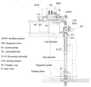
Figure 3: The U400R axial injection
