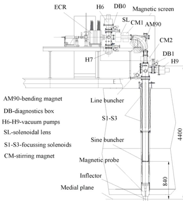
Figure 4: The sketch of the U400 modernized injection
